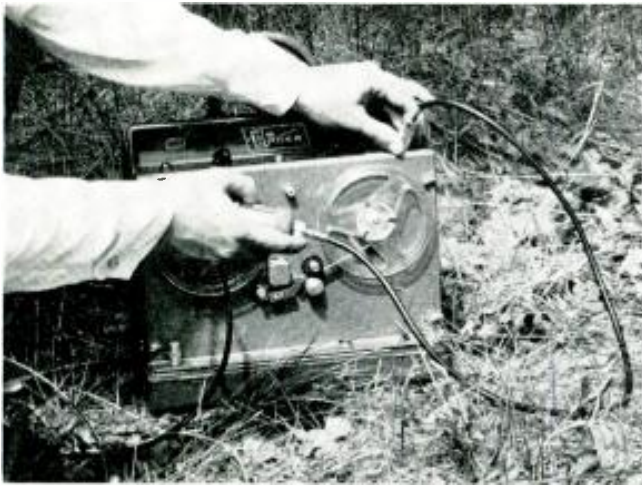
If you must run a long line, a microphone transformer should be used to match the impedance of the mike to the input impedance of the recorder. A low impedance mike and low impedance cable are best. If a high impedance mike is used, two transformers and a low impedance line are necessary.
