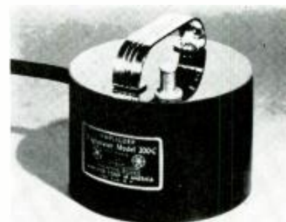
The Magneraser, a handy bulk eraser is used to wipe tapes clean for the next recording. The unit is plugged into the regular 110 volt line and brought into contact with both sides of the reel. It may also be used to demagnetize heads.
