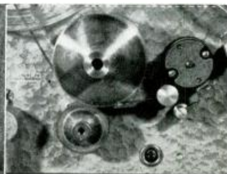
Tape threading is easy and straightforward, and should be done before the flywheel is put on. The reversible head can be seen at the right.
