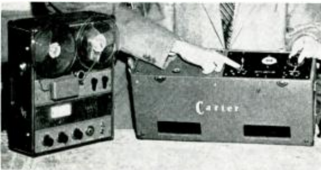
A new power pack, just brought out by Carter Motors, supplies the necessary current for tape recorder operation. It features a 12 volt battery which operates an inverter to deliver the necessary 110 A.C.
