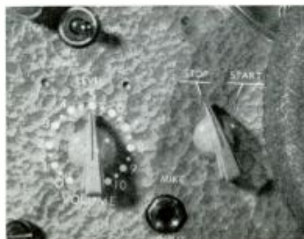
To the left is the volume control and to the right the start and stop switch. The microphone input jack can be seen below the control knobs.
