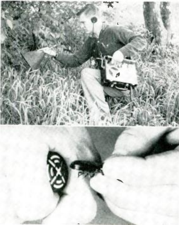
Top: the author preparing to record a ground cricket with the mike fastened inside a household funnel to eliminate extraneous noises. Lower: recording the "protest" note of a Passalid or Betsy Beetle. This insect makes its noise with its tail end, by rubbing two sharp projections on its abdomen against the undersurface of its wings.
